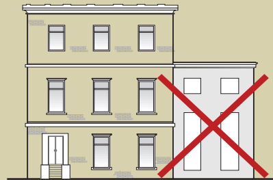
Floor to floor height should be similar.
