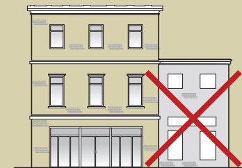
Windows and doors should have a similar size, shape, scale, and proportion.
